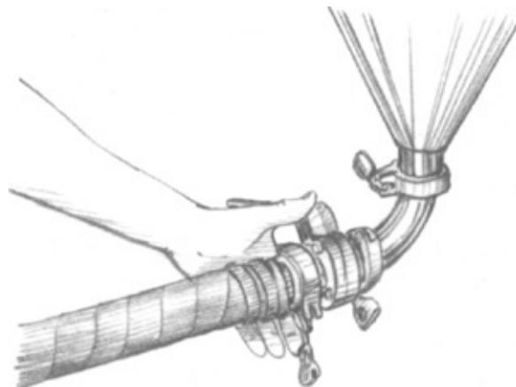
*Connecting a hose to a flange with a triclamp is a simple procedure — much easier than traditional plumbing connections.*
