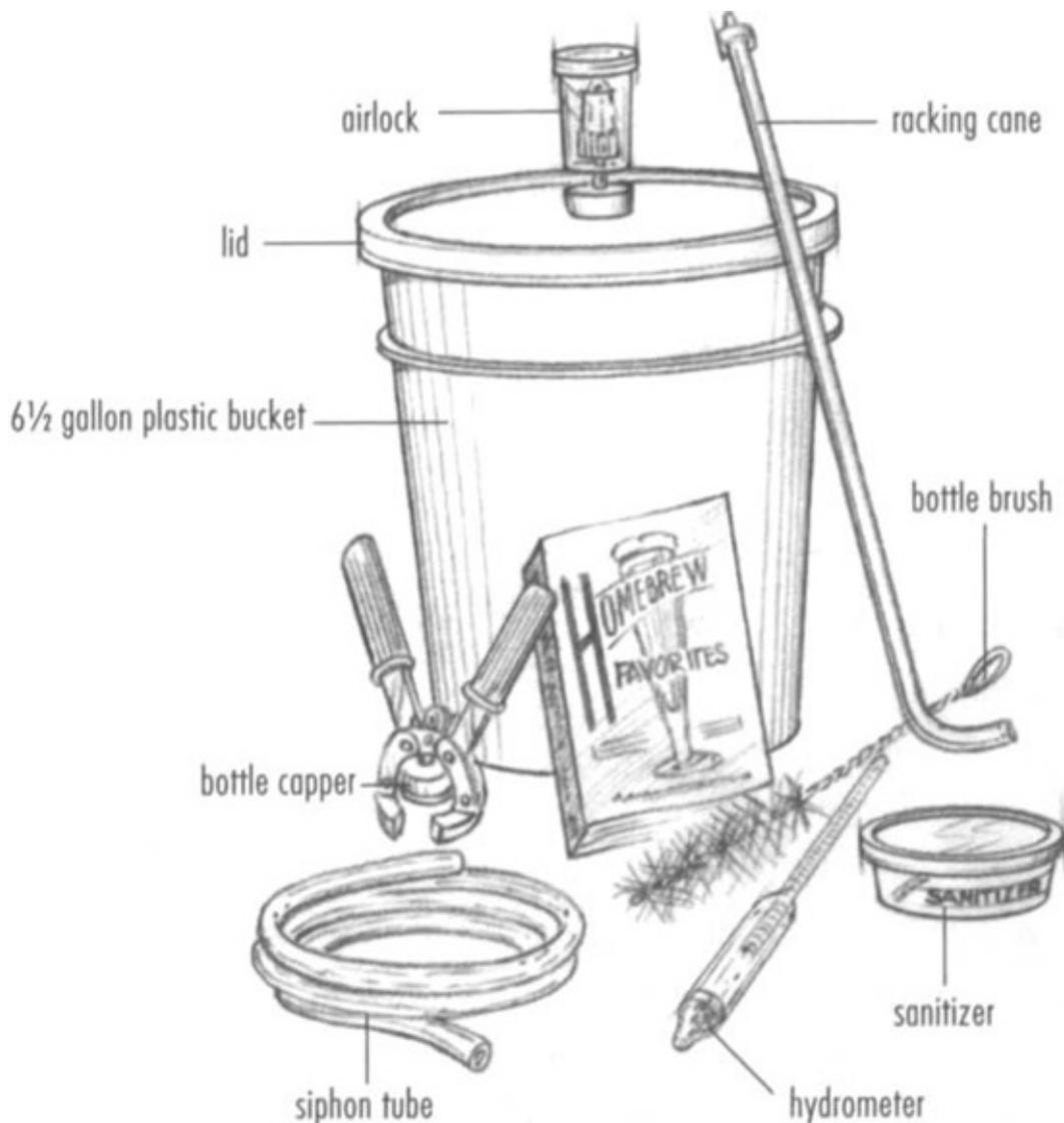
*Basic homebrew equipment should include: a plastic bucket and lid, a hydrometer, a*
