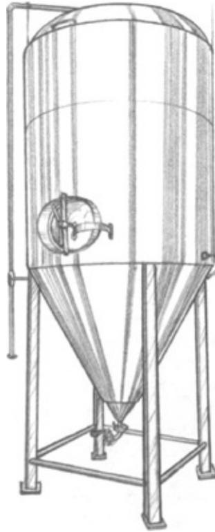
*Cylindroconical fermenters, such as this one at Brimstone, circulate refrigerated glycol to reduce the heat and maintain the proper temperature.*
