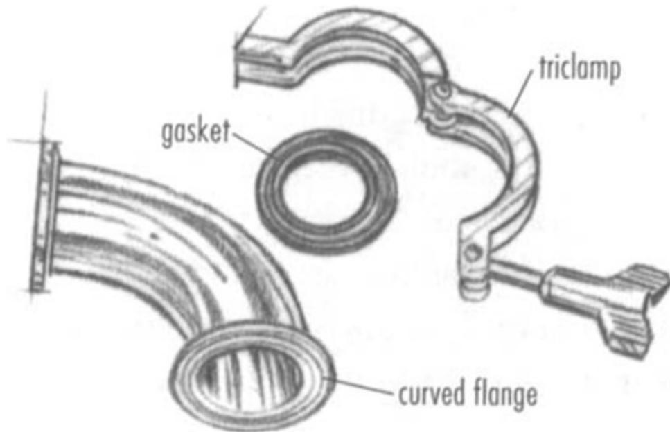
*Professional brewers use quick-disconnect fittings such as this triclamp, pictured here with a gasket and flange, to keep the process flexible.*
