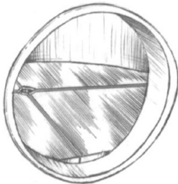
*False bottoms are common in commercial small breweries. The slotted false bottom allows sweet liquid to drain across the entire area of the bottom of the grain bed.*
